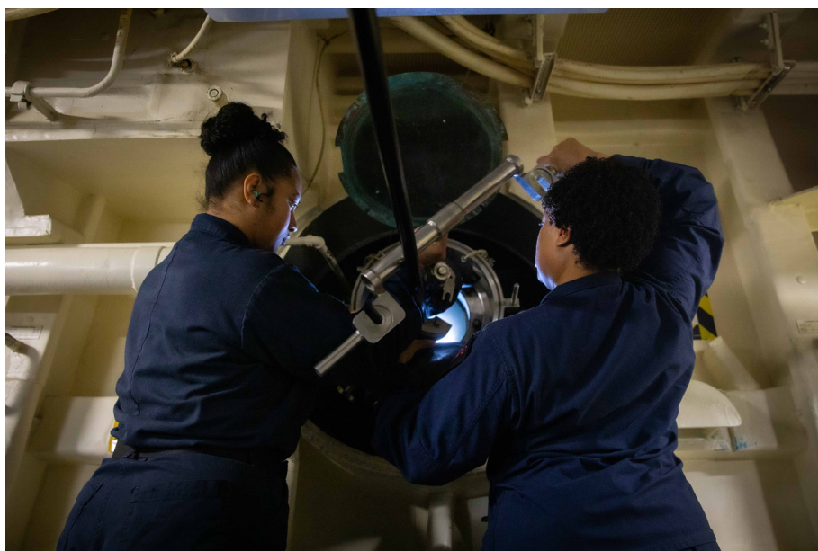
U.S. Navy Sailors assigned to the Arleigh Burke-class guided-missile destroyer USS Paul Ignatius (DDG 117) deploy a multi-functional tow array (MFTA), Mar. 5, 2024.
